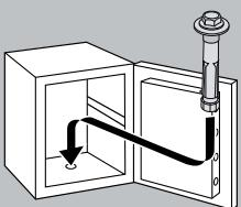
GB The safe must be anchored before being use.
