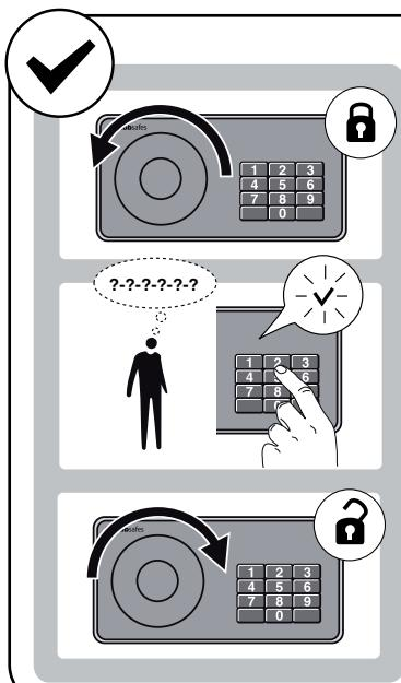
GB Check that your PIN code has been retained. Operate the lock three times without closing the door. If not, reset your PIN code.
